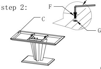
Connect Table top frame(C) to Stainless steel pillar (B) with bolts (F) (M8\*60), Tighten
