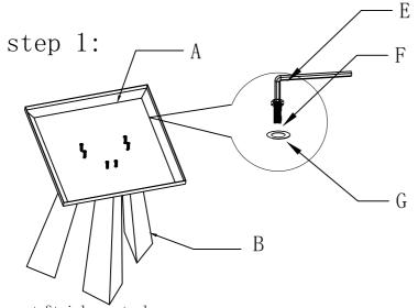
Connect Stainless steel pillar (B) with Stainless steel base (A) by Screw (F) (M8\*30), tighter, one by one
